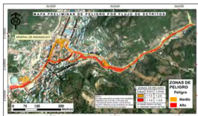
Figure 3. Debris flow hazard map for Angangueo. Obtained with numerical modelisation using FLO-2D (Figuroa-Miranda, 2013).
