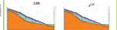
Fig.4 FOS and critical slip surface using limit equilibrium method (left) and the finite element stress method(right) in static state
